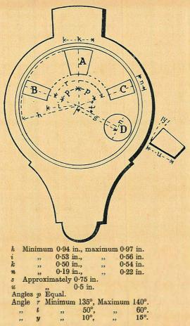
Shutter.—The lid shall be equipped with a brass shutter, approximately 0·1 in. (0·25 cm.) thick operating on the plane of the upper surface of the lid. The shutter shall be so shaped and mounted that it rotates on the axis of the horizontal centre of the lid between two stops so placed that when in one extreme position the openings A, B and C of the lid are completely closed and when in the other extreme position these orifices are completely opened.
